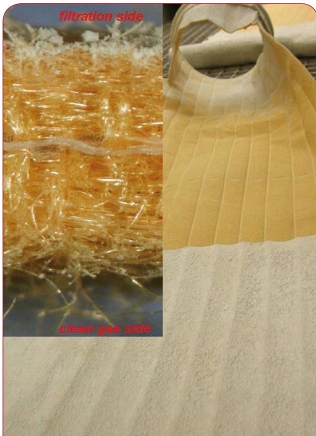
Figure 3. P84 needle felt on PTFE scrim after two years at 185 °C (peaks up to 230 °C) in an alkali bypass filter.
