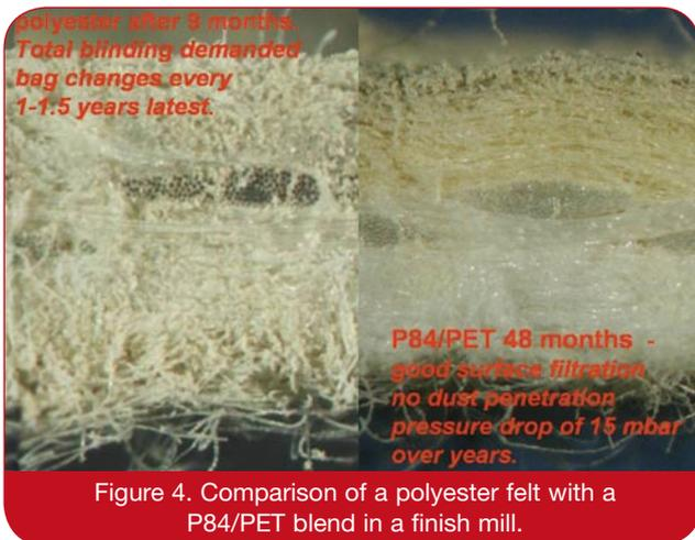
Figure 4. Comparison of a polyester felt with a P84/PET blend in a finish mill.
