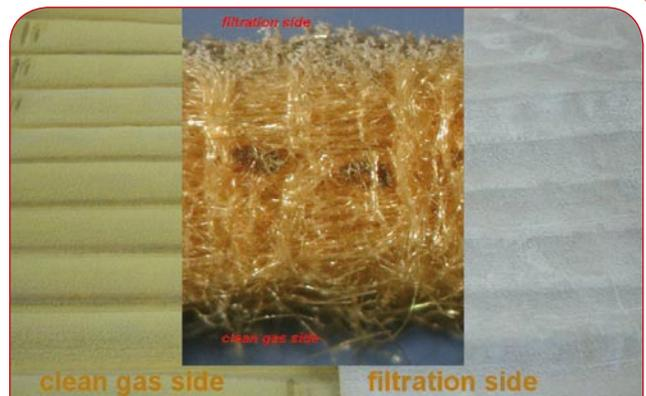
Figure 1. P84 needle felt on a P84/PTFE hybrid scrim after eight years in a kiln filter in Brevik/Norway.
