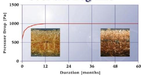
P84 needle felt on a P84 scrim in a kiln filter. Excellent filtration behaviour and sufficient mechanical stability for 6 years bag life (1,2 m/min at 165 °C).
