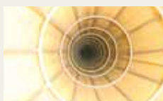
View inside a P84 based filter bag
