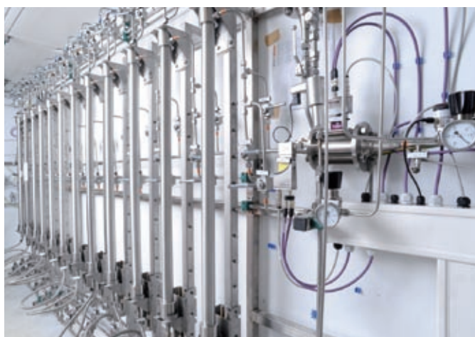
Multi-staged membrane modules, dedicated to the needs of biogas upgrading
