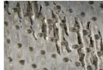
Damaged membrane surface after 29 months
