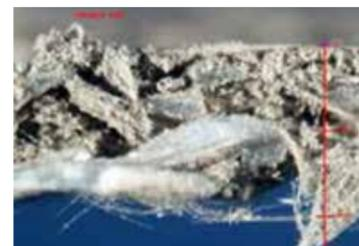
Dust contaminated cross section of a glass fabric as a result of membrane damage
