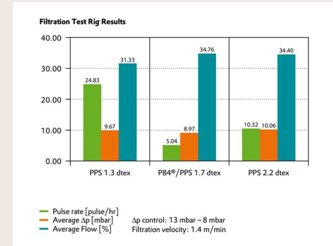
The above diagram shows the results of a comparative testing of 3 different filter media. Two of them are based on PPS fibres. The third contains P84® fibres to increase the filtration performance. As a result, the filter bag containing P84® shows the lowest pulse rate and pressure drop compared to the other bag materials in the test.
