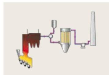
The main benefits are a low and stable residual pressure drop and long filtration cycles. High collection efficiency is achieved for fine particulate also. This ensures low emissions and an efficient use of the absorbent.
