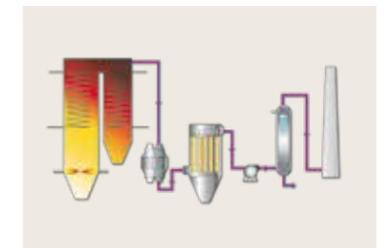
When using biomass, the operation load of the plant varies in a wide range. Operation at low boiler load sometimes causes high values of unburnt hydrocarbons and temperature fluctuations.
