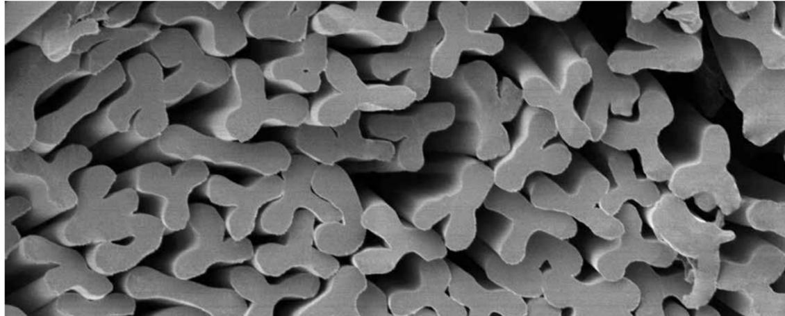
The P84® fibre is a polyimide based fibre with a typical textile character. Polyimides are known to be used in a wide range of operating temperatures starting from cryogenic applications and ending at high temperature applications at the limits of polymer based materials.
