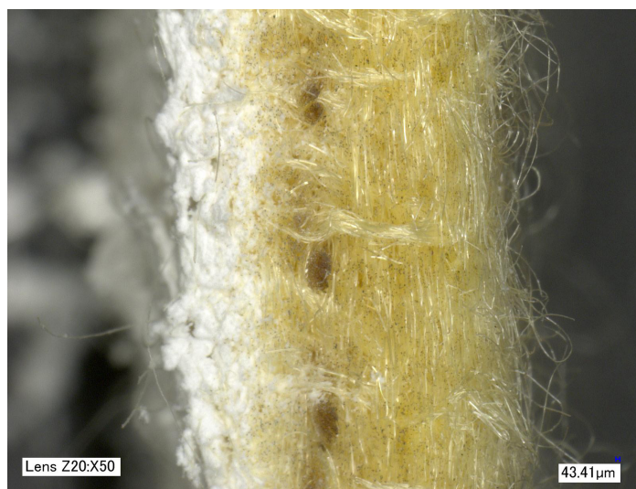
Figure 5. P84 microfibre cap after VDI test.
