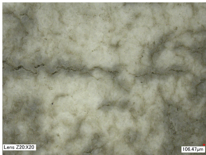
Figure 3. Submicron particles damage e-PTFE membrane.
