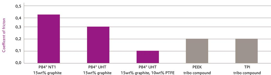
$F_N = 250 \text{ N}$ ,  $v = 1 \text{ m/s}$ ,  $23^\circ\text{C}$ , 20 hrs, counterpart: 100Cr6, bearing dimension: inner diameter = 30 mm, outer diameter = 34 mm; no lubrication
