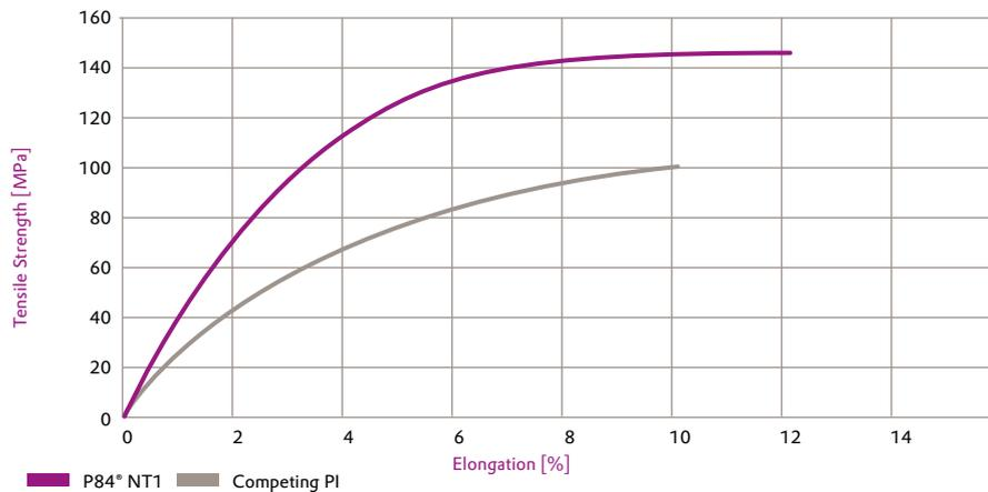
Comparison of stress-strain-curves in tensile test (ISO 527). Polyimide P84® NT shows a wide area of elastic behaviour and high mechanical stability.
