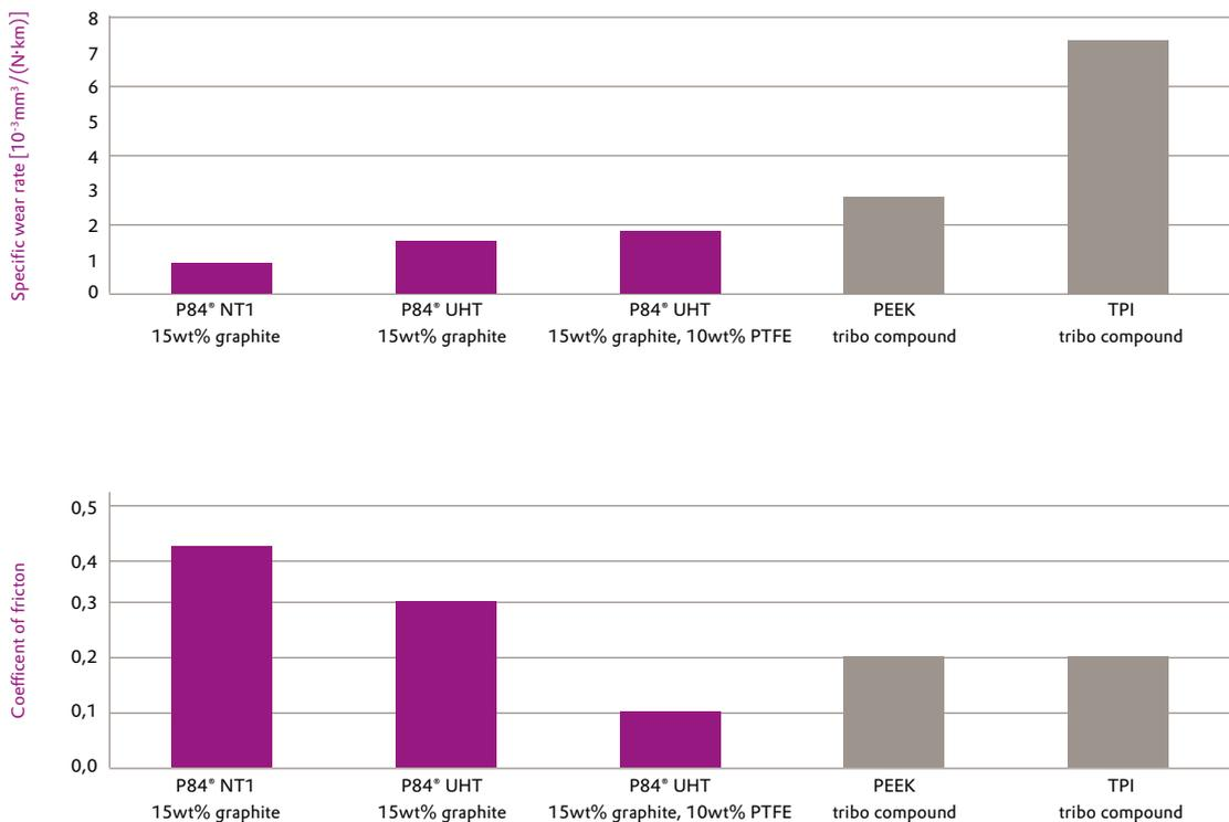
$F_N = 250 \text{ N}$ ,  $v = 1 \text{ m/s}$ ,  $23^\circ\text{C}$ , 20 hrs, counterpart: 100Cr6, bearing dimension: inner diameter = 30 mm, outer diameter = 34 mm; no lubrication
