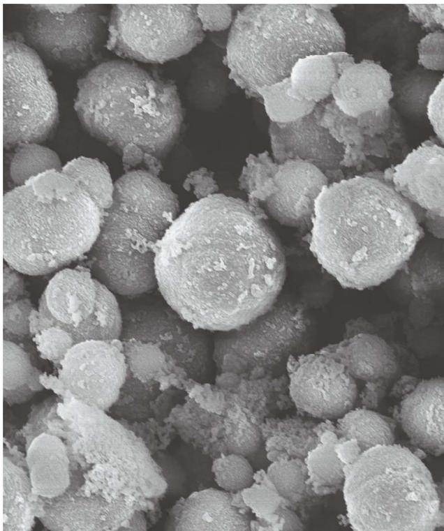
Scanning electron micrograph (SEM) at 4000× magnification. Spherical particles of Polyimide P84® NT with smooth surface.
