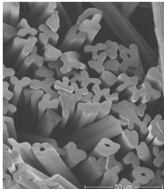
Fig. 1: Multilobal fibre cross section of P84®
