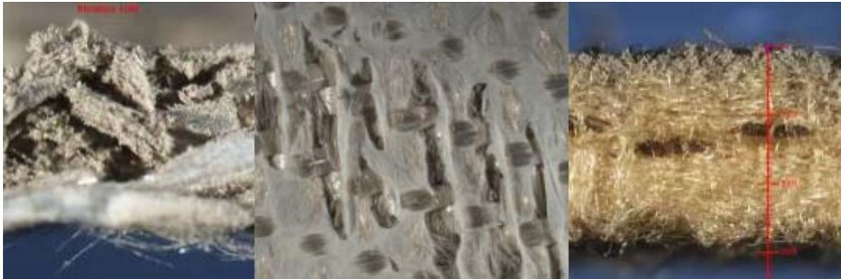
Fig. 3: cross section of filter media after 29 months operation; from left: glass with e-PTFE-membrane; cracks on the membrane surface; dust-free cross section of P84®
