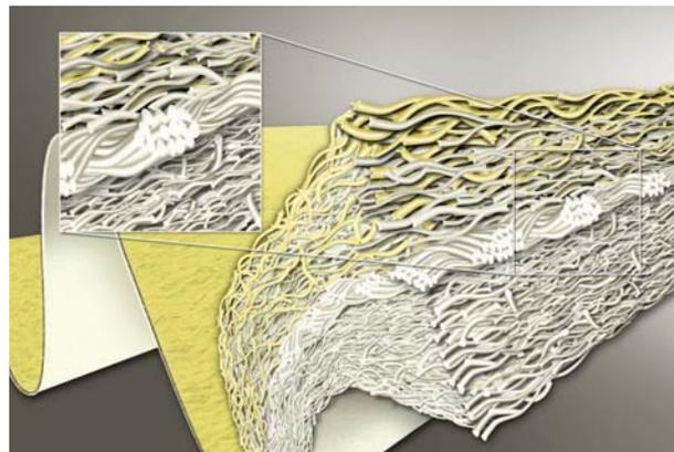
Fig. 5: Illustration of an asymmetric P84®-blend
