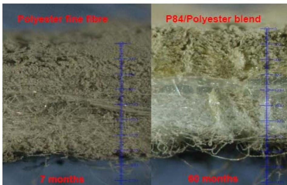
*Fig. 6: Finishing mill: Polyester fine fibre felt after 7 months (left, total blinding - the bags had to be changed) in comparison with a P84®/Polyester blend after 60 months in operation (right, constant pressure drop of app. 1500 Pa). See tab.2 for details*
