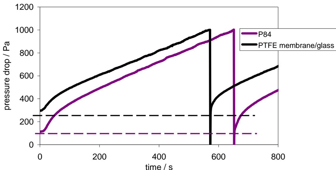
Fig. 4: Pressure drop development of kiln filter media after 29 months operation, evaluated on a test rig according to VDI 3926
