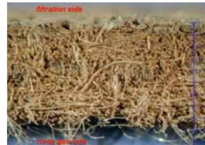
Blinding of a PET felt in the same installation
