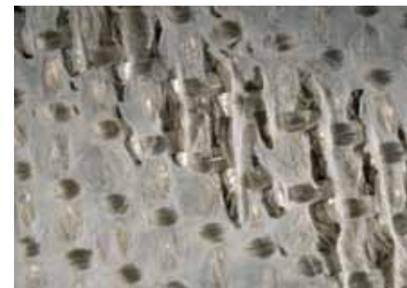
Damaged membrane surface after 29 months
