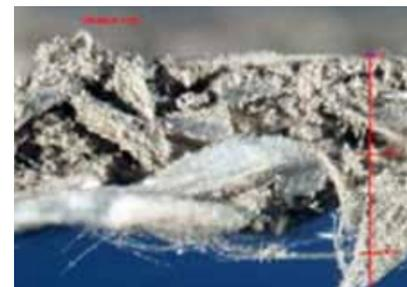
Dust contaminated cross section of a glass fabric as a result of membrane damage
